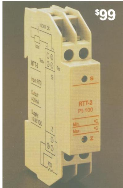
Ambient Temperature Range: -4 to 158°F (-20 to 70°C), 5-95% RH Storage Temperature Range: -22 to 185°F (-30 to 85°C) Enclosure: polycarbonate, IP40 protection Terminal Housing: polycarbonate, IP20 protection Mounting: 35 mm DIN rail Dimensions: 3.54" H x 0.7" W x 2.28" D (90 x 17.5 x 58 mm) Weight: 2.5 oz (70 g)
